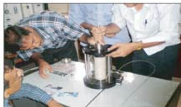
Triaxial Test is being conducted
