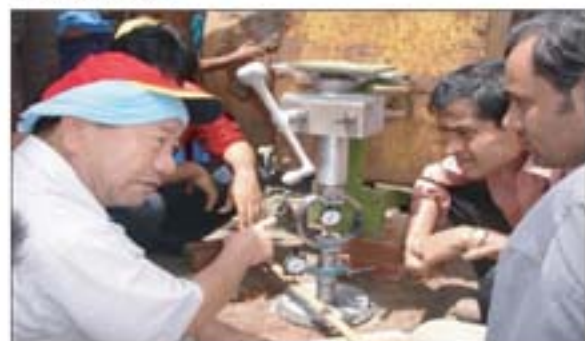
Field CBR Test is being conducted in the laboratory
