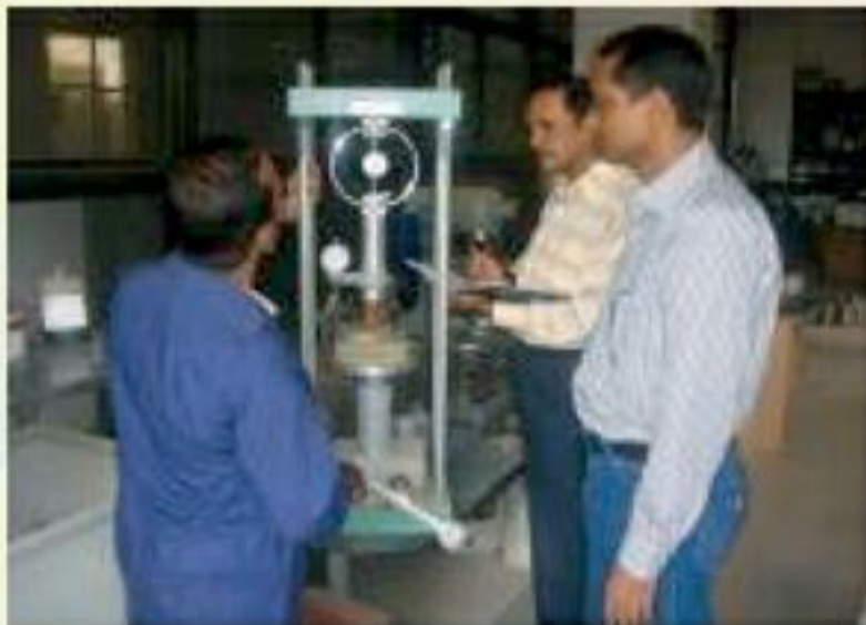
Soil testing by Unconfined Compression Test method being done in the laboratory
