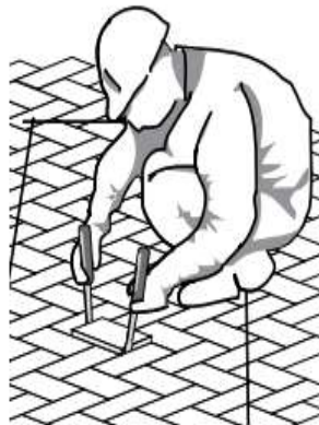
Figure 3. Prying the paver upwards with two large screwdrivers.
