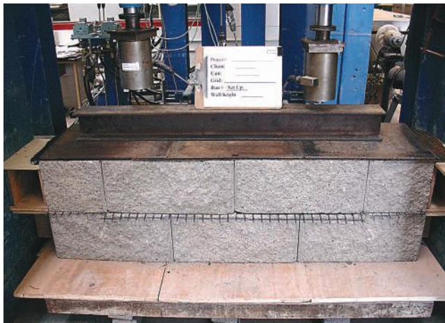
Figure 19. Geogrid connection testing with SRW units
