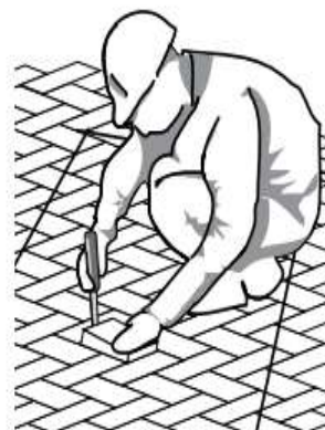
Figure 4. Prying with a screwdriver and pulling the paver out.
