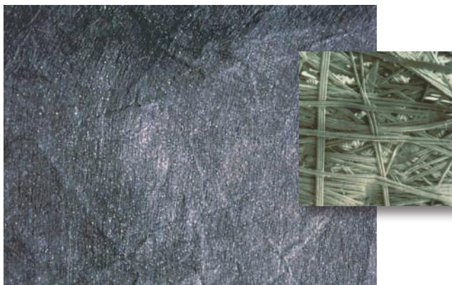
Figure 15. Non-woven heat bonded geotextile with close-up
